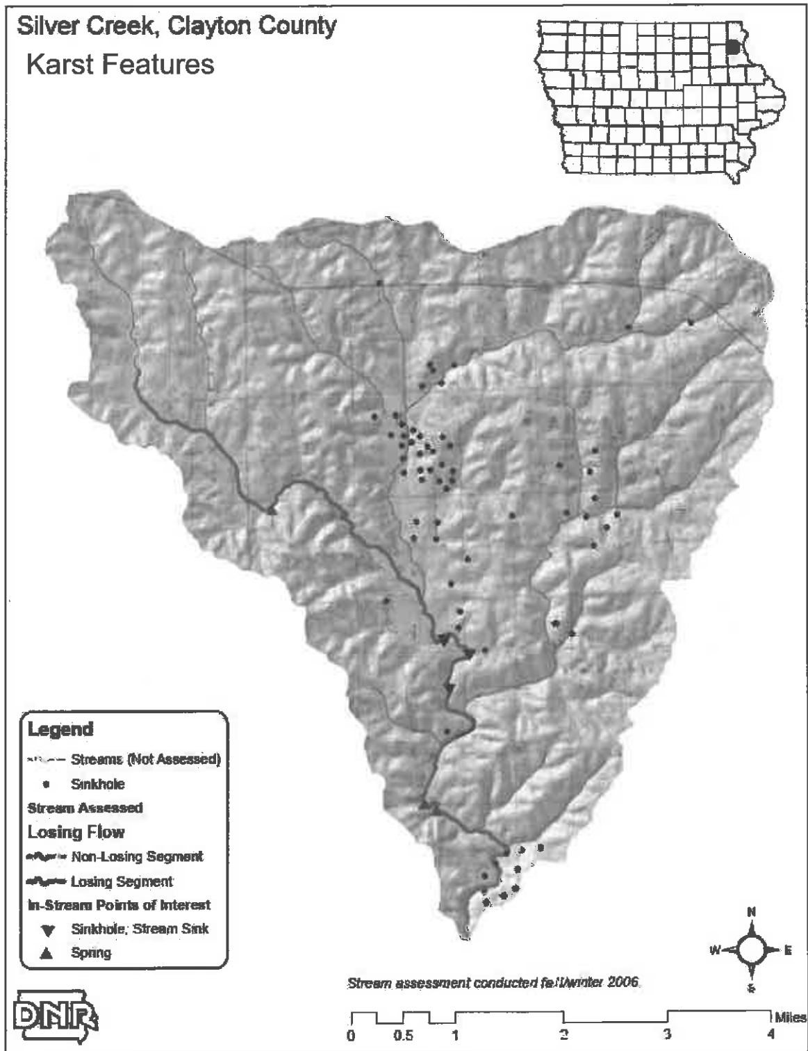
Figure 2-3. Locations of springs, sinkholes, and in-stream sinks in the Silver Creek watershed.
